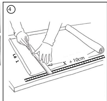
④ Crop the image according to your preference, either from the top or from the bottom, cutting off the excess (leave yourself a safety margin).
