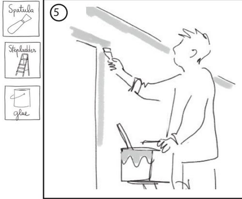
5 The sensitive parts of the wall need to be glued: wall, door frame/top and bottom edges.
