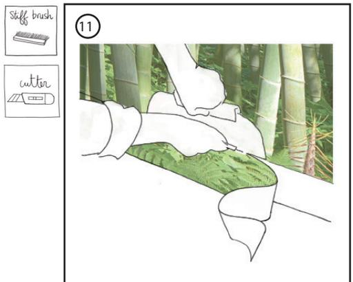
11 Cut off the excess with a cutter using the spatula (be sure to use a new blade).
