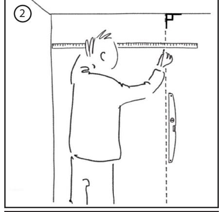
② Measure the width of the first strip. Use a level to draw the dotted lines.
